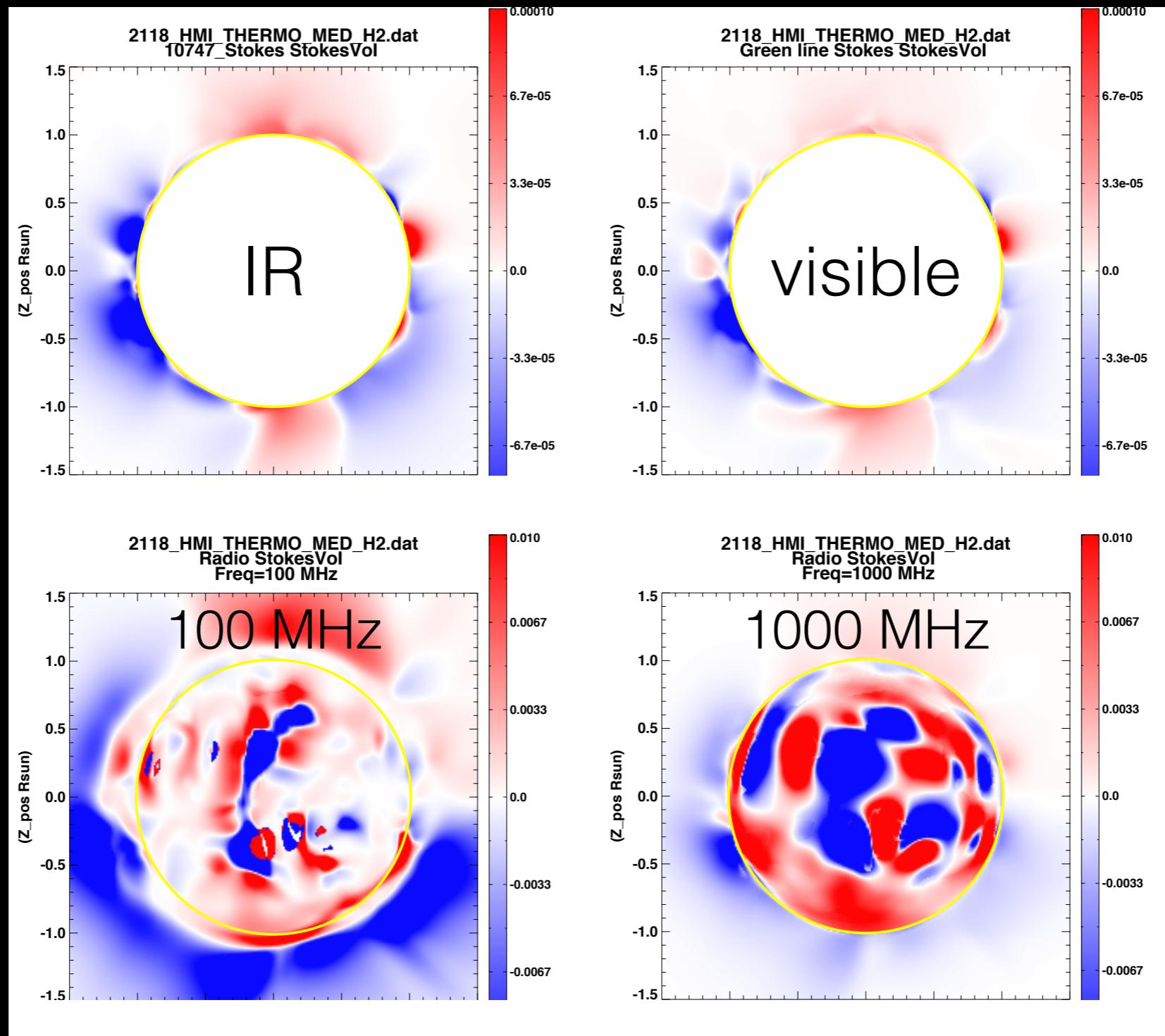
**Circular polarization at different wavelengths:
